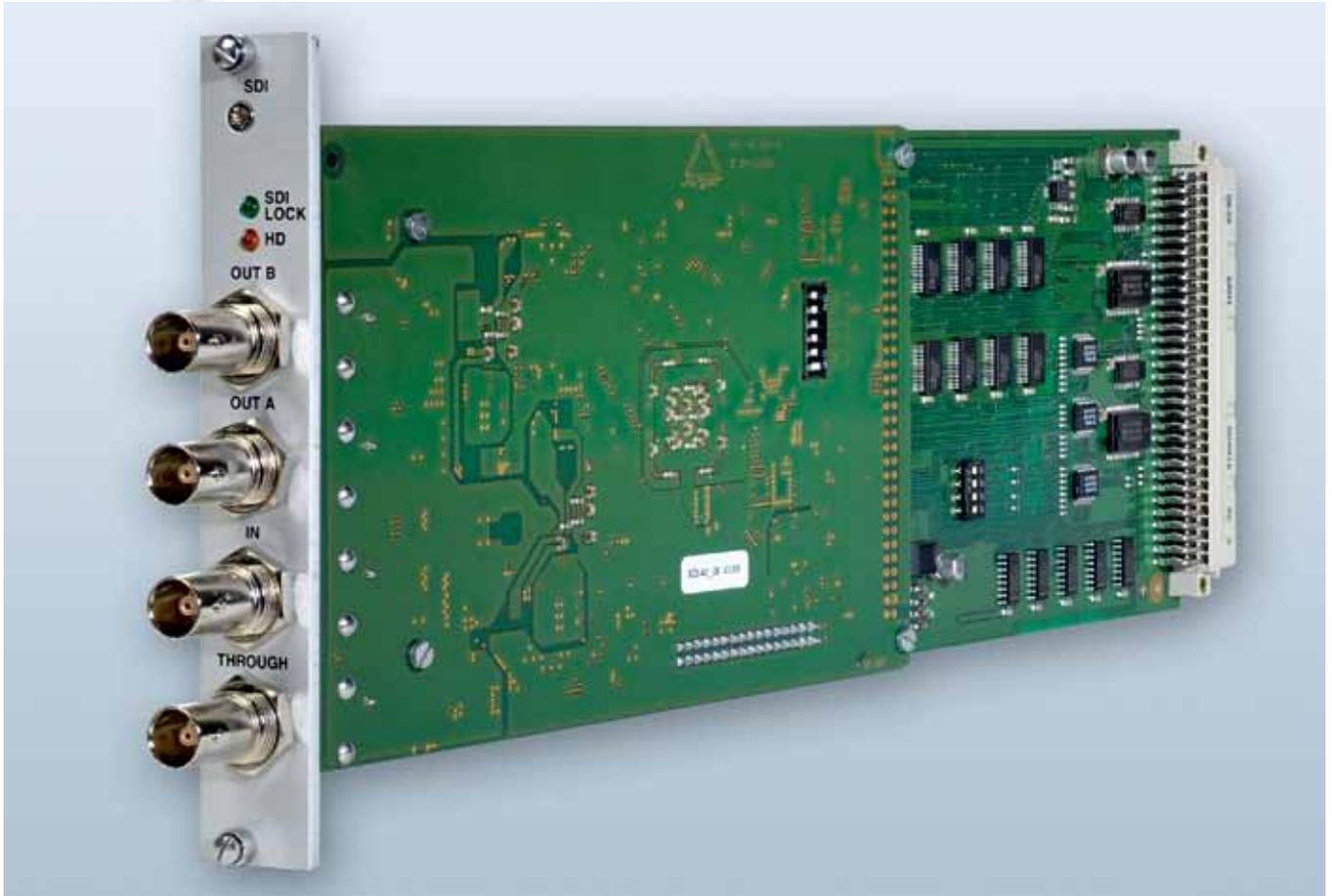
The SDI Card is an option card available for the Studer D21m I/O system, and allows the de-embedding of the audio stream from an SDI (Serial Digital Interface) signal.
