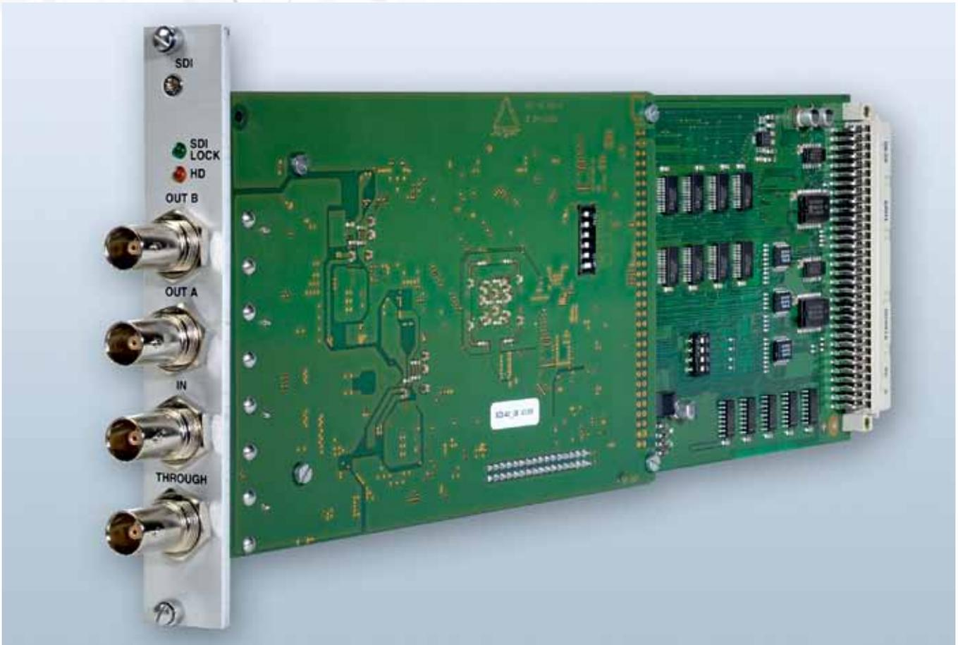
The optional 3G/HD/SD SDI (serial digital interface) embedder/de-embedder card is able to handle video signals according to the 3G (full HD), HD and SD standards; both level A and B versions of 3G signals are supported. Standards selection is performed automatically.
