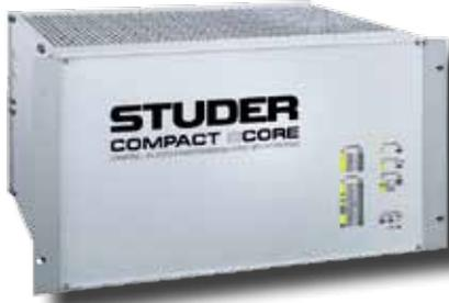
Housed in a 6U frame which can be equipped in the upper part with up to six DSP cards, the controller card, time and clock synchronization interfaces and GPIO cards, the Compact SCore provides I/O capacity up to 576x576. The lower 3U part includes the standard D21m I/O system.
