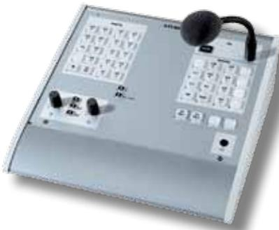
The Monitoring and Talkback Box for Studio 2 and Studio 3 have a reduced feature set offering an array of configurable buttons for monitoring source selection and talkback destinations, red light indication, studio loudspeaker and headphone control and connection.
