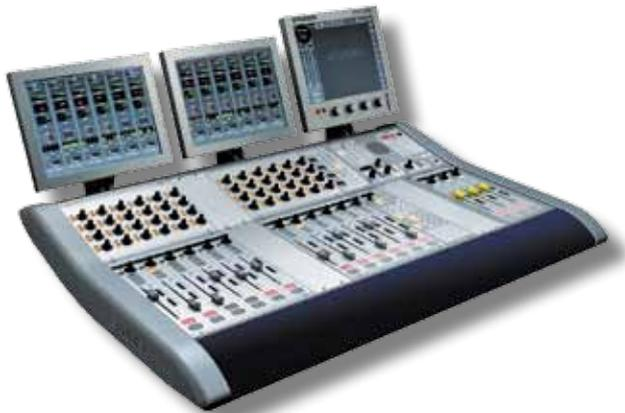
*Example of a fully equipped console with 12 channel faders, including Rotaries, Assign modules, Fader Screens, Monitoring and Talkback, Master Screen and a 3 fader Master section, e.g. used for the three main output buses. In general it is quite possible to assign any master bus to any fader on the console or as another example to use a 6 fader module for group faders or AUX master bus controls.*
