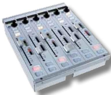
Every fader strip includes five illuminated keys, the fader, an LED input level meter which may be set for AF/PF and N-X send level, with overload indication, an LED gain reduction meter, and an 8 digit alphanumeric channel label display.
