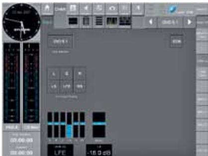
The 5.1 Input Channel has its own Input Routing setup accessible from the User GUI, where any configured physical Input can be routed to any of the 5+1 individual Channels.
