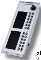
The XL Module enables direct communication to up to twelve outside sources. It features 12 eight digit alphanumeric displays for source label indication, 12 buttons each for PFL of and TB to these individual destinations and a rotary control for individual and sum volume control. In a typical application during, for example, a sports event or election communication where many outside locations need to be controlled, the XL Module is a fast and ergonomic solution.
