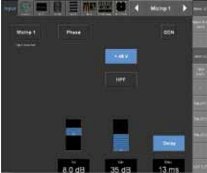
To compensate for audio to video signal offsets when operating the OnAir 3000 in a TV environment, systems using the SCore Live DSP core enable a delay function. During operation, delay can be activated on input channels, master and aux busses, N-x and subgroups. It is possible to set any delay time between 0 and 5 seconds in a resolution of milliseconds.
