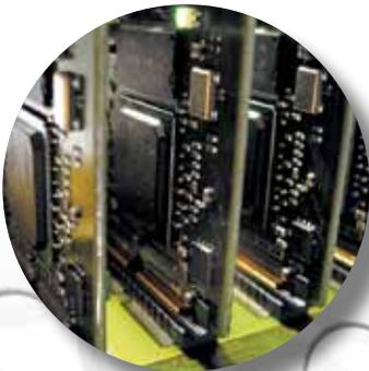
The audio data is processed with a resolution of 40 bit floating point guaranteeing absolute Studer high end audio quality. The SCore and consequently the OnAir 3000 use the same DSP audio algorithms, e.g. for equalisation and dynamics, as are used in the large frame Vista and D950 mixing consoles resulting in unparalleled Studer audio quality.
