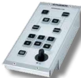
The Surround Control Module is an extension to the existing Monitoring and TB Module. The user can easily switch between Internal Stereo Mixdown and External Stereo Encoder (e.g. DOLBY®), mute individual speakers and switch to an alternative Stereo Nearfield speaker set with its own dedicated volume control rotary.
