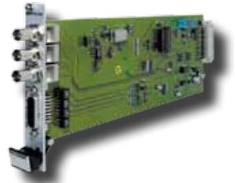
The Clock Synchronisation board allows the internal clock frequency of the OnAir 3000 to be synchronised to an external master clock. Synchronisation to the following external signals is possible:
