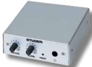
This headphone amplifier can be fitted on top or under the table with respective mounting brackets. It can be connected directly to a line output of the D21m I/O system and features a local amplifier with volume control. In addition a talkback signal with separate volume control can be enabled and brought to the guest headphone, heard in split mode and controlled via a GPO signal.
