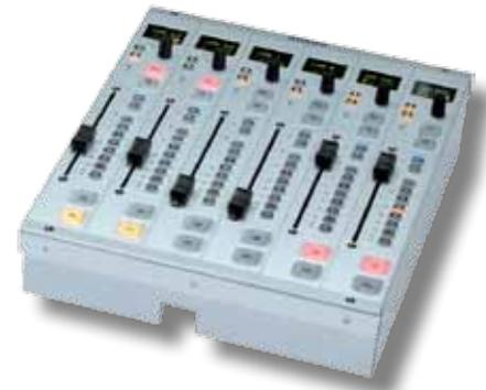
The module contains 6 full 100mm faders, 4 large illuminated and configurable pushbuttons with replaceable label, and 12 small illuminated pushbuttons per channel. Two LED's in each fader strip indicate channel overload (red) and active fader start (blue). Level and gain reduction meters are shown on an OLED display on every channel.
