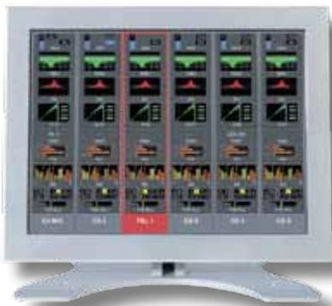
The colour 12" touch sensitive fader screens display the input settings, equalizer and dynamics settings, AUX send levels, N-X contribution, input, output and insert routing, bus and group assign, Pan/Bal and channel label, all in real time with real values.
