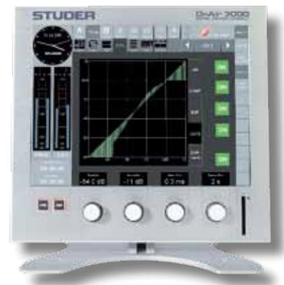
The screen includes a studio clock, two stereo bargraph meters each with phase correlators, two stop watches, menu buttons and eleven freely assignable buttons on the right border of the screen. These buttons can be used in the same way as the buttons in the Fader Assign Module.
